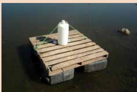
Jain Aqua Saver mounted on the float
